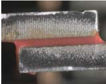
Photograph of lapjoint showing the adhesive yielding and cracking around adherend end radius
