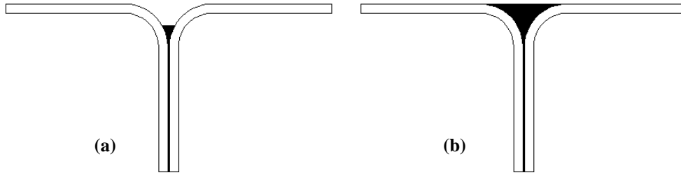
Figure 5 - Schematic of the T-peel joint with (a) 50% resin fillet and (b) 100% resin fillet
