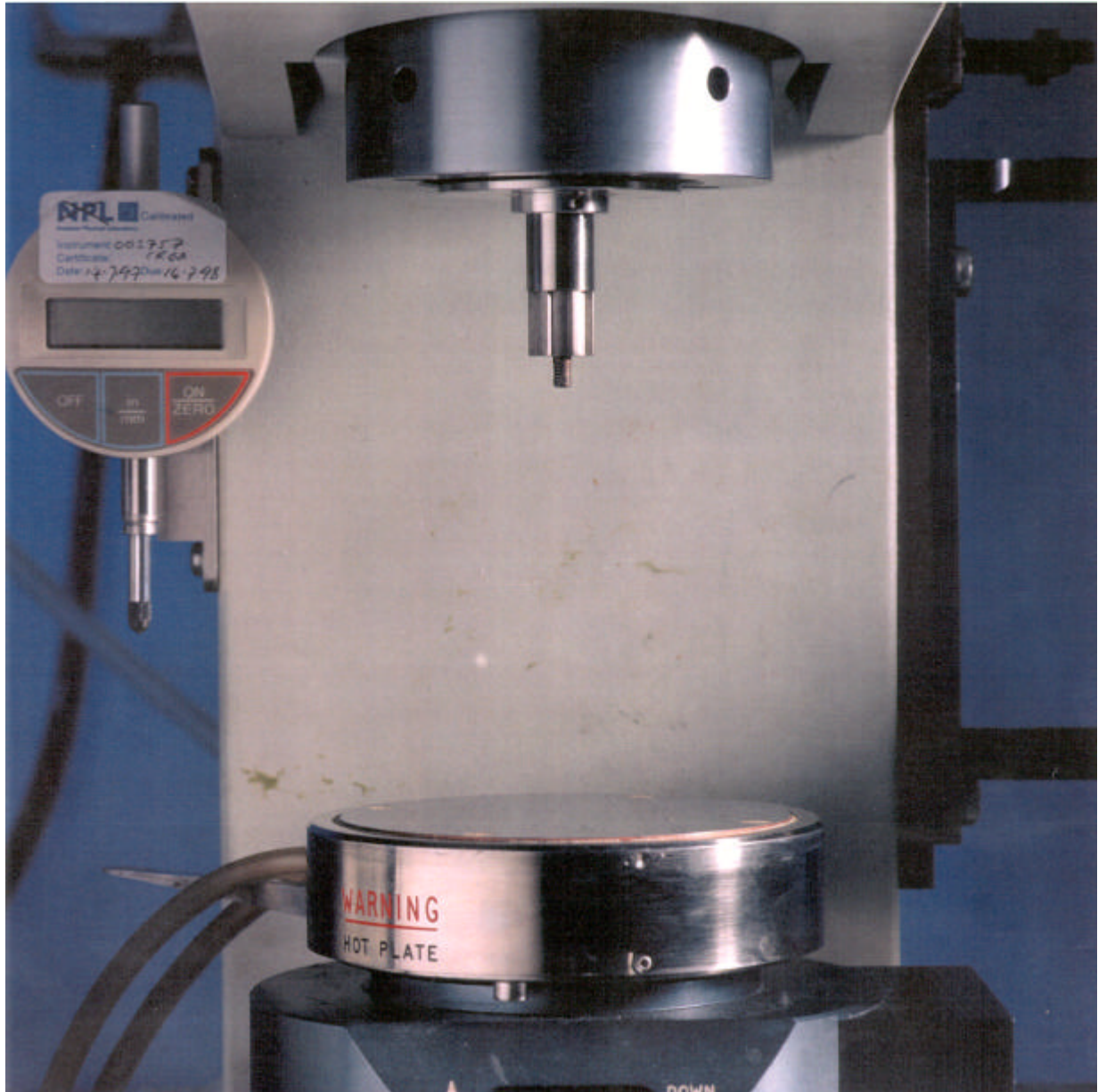
Plate 3: Close up of CSL 2 500 modified air bearing
