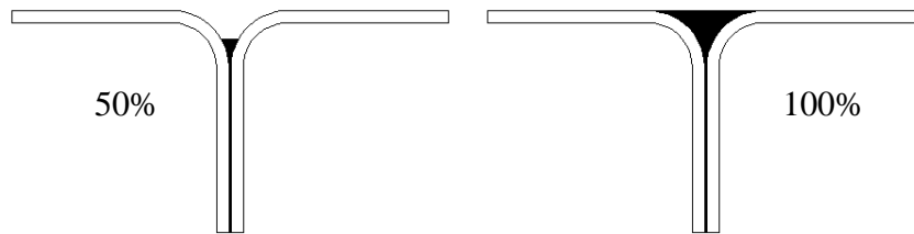
Figure 3. Schematic of the adhesive fillet geometries for the T-peel joint.
