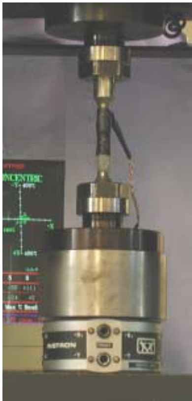
Figure 2: An accurate alignment fixture improves the reliability of the butt-joint test data.
