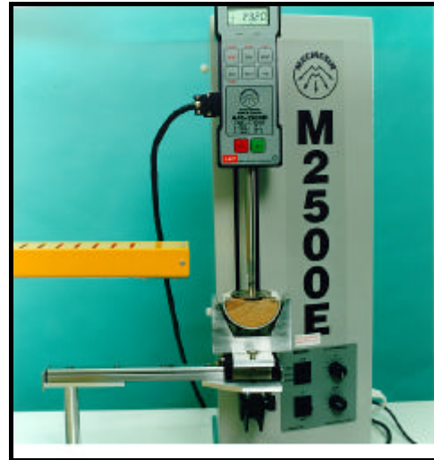
Figure 2: SATRA/NPL Shoe Tack Tester
