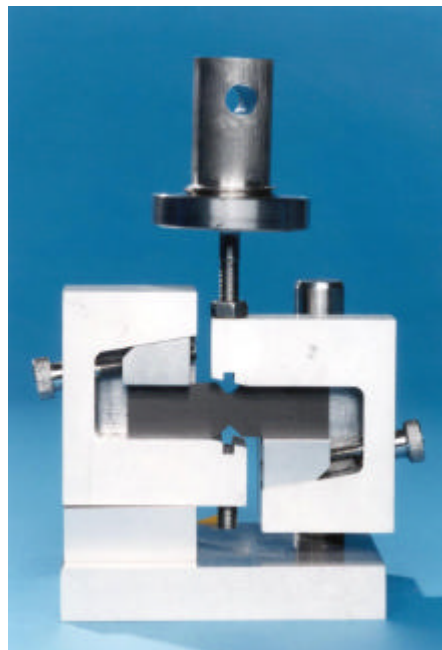
Figure 1: V-notched beam test fixture and specimen
