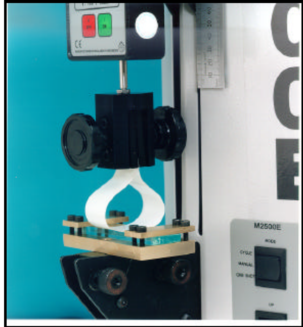
Figure 3: Full Contact is Obtained in a FINAT FTM 9 Test
